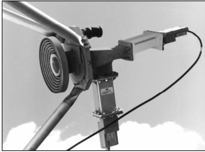
7893D mounted between antenna feed & LNA (both Vertical & Horizontal Polarization)
