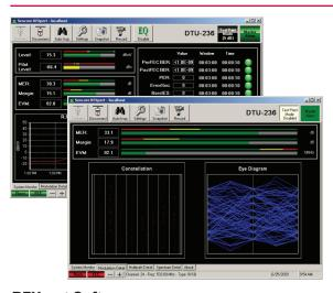
The DTU-236 can be combined with Sencore's RFXpert software for a truly powerful RF measurement tool. RFXpert provides easy-to-read spectral displays, both constellation and eye diagram displays, and the ability to turn off and on 8-VSB tap equalization to see the uncorrected signal being received.
