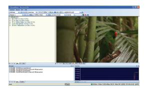
Adding StreamXpert to a DTU-236 makes for a cost-effective and user-friendly MPEG-2/H.264 transport stream analyzer. Signals can be analyzed from either the ASI or RF inputs of the DTU-236 and can be validated against industry-standard ETR101-290 templates. Transport streams can also be captured in the field with StreamXpert for later use.
